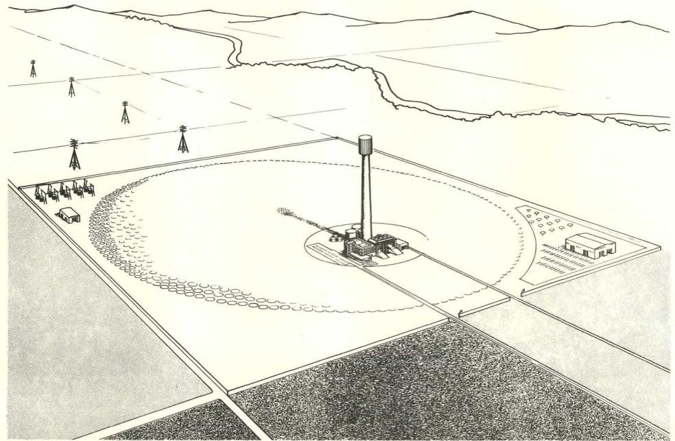
DRAWING of 10-megawatt solar-powered pilot plant shows central receiver (the tower), surrounded by fields of heliostats that redirect solar radiation to the
